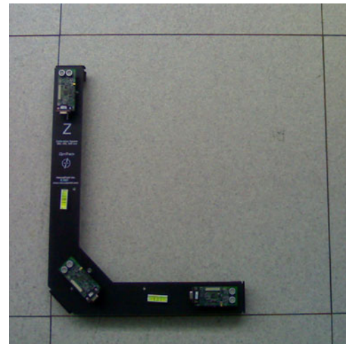
Fig. 4 Reference artifact prototype. In this case the number of devices embedded is three
